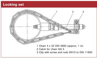
Locking set for push-in sensors. Ordering no.: 0Z122Z000204
