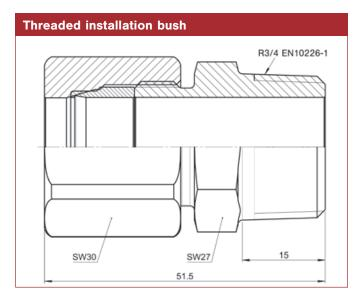
Suitable up to 25 bar/363 psi abs. if used with push-in sensors. Please observe assembly instructions and safety guidelines! Metal sealing ring can't be disassembled after assembly.
