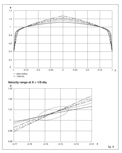
Max. accuracy is achieved with an insertion depth of x = 1/8 inner pipe dia. (fig. 7).
