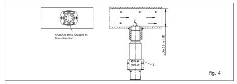
With inner pipe diameters of > 56 mm the middle of the probe (chamfer) must be screwed in to 1/8 of the inner pipe diameter.
