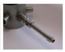
The push-in type process connection is used for bigger pipe sizes (> 2'' / > DN50). The push-in type sensor is pushed through a special threaded installation bush (order number VK-04D8M1).
