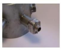
The screw-in type process connection is the standard connection and available for every sensor. The customer just has to weld a ½" sleeve to the pipe and then screw in the sensor. 螺丝旋入式工艺连接是标准安装连接,每个传感器都可以使用。客户只需要焊接½"套筒的螺旋管然后再拧进传感器。
