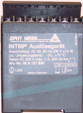
Fig. 20: PTC thermistor release device INT69
