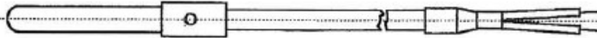
Figure 14: Metal sheathed thermocouple, extension grade wires attached (can also be delivered with thermal plugs)
